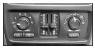
(Fan): Turn the left knob clockwise or counterclockwise to increase or decrease the fan speed. If the knob is in off mode, outside air will still enter the vehicle, and will be directed based on the position of the mode knob. The temperature can still be adjusted using the temperature knob.
